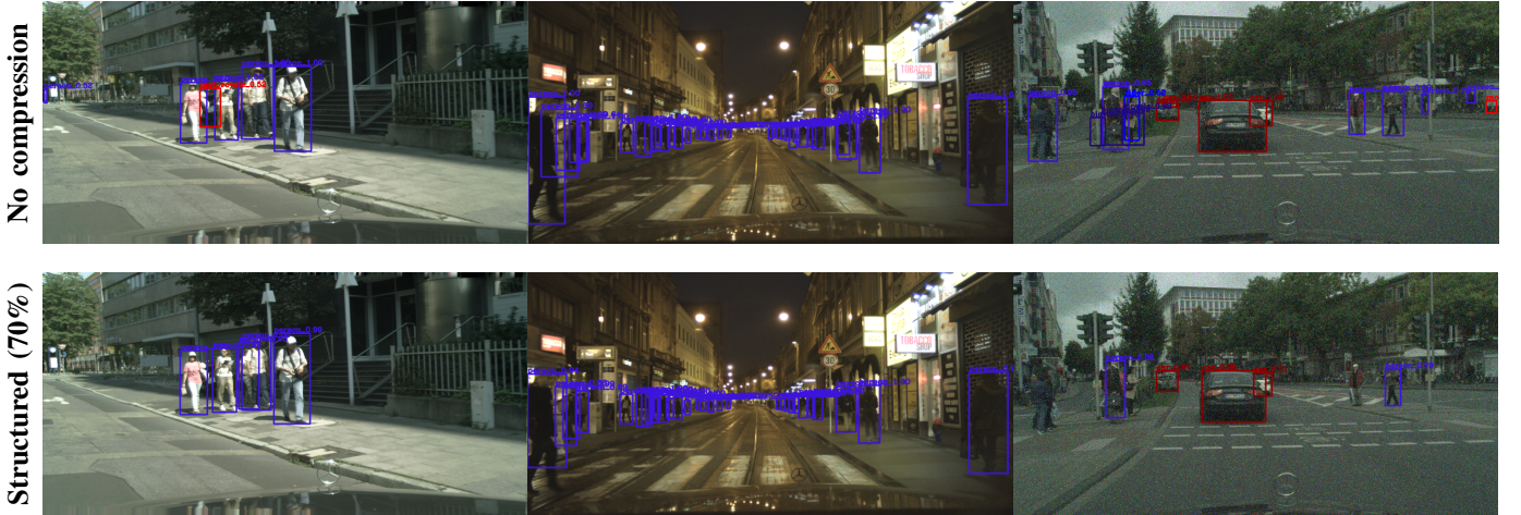
Fig. 5: Detection samples for base model and the model structurally pruned at 70% compression rate. Detections on the original Cityscapes dataset (first column), ECP dataset (second column) and noise distortion (third column).
