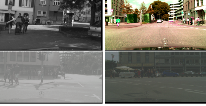
Fig. 1: Examples of augmented images: color drop (top left image), color distortion (top right), overexposed image (bottom left), gaussian noise (bottom right).
